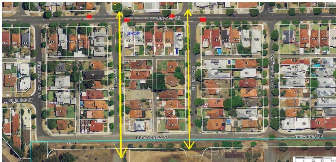
Anzac Road is classified as a District Distributor B in accordance with the Metropolitan Functional Road Hierarchy, has a posted speed limit of 50 kph, and provides a link between Oxford Street and Brady Street. The 85% speed is about 9 kph above the posted speed in some sections of the road. The Police have in past deployed traffic officers to monitor and enforce the 50 kph speed limit both as a visual deterrent and to change driver behaviour.
