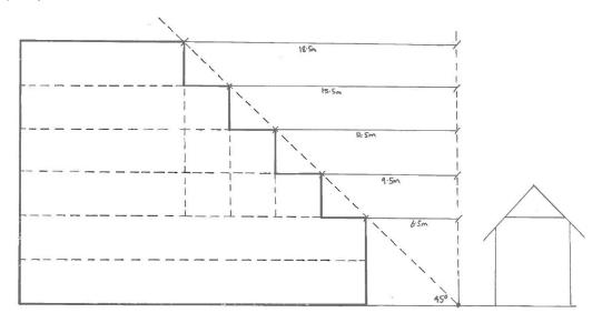
Figure 1: 45 degree angle approach to setback calculation
