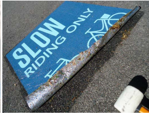
Bottom edges lifted after application
