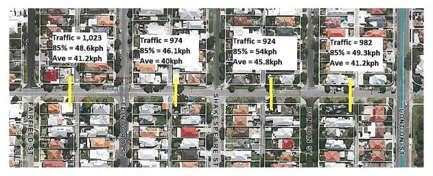
As part of the Shakespeare Street Bike Boulevard project, a raised plateau is being installed at the intersection of Shakespeare and Ellesmere Streets and the existing stop control on Shakespeare Street will be changed to a give way control on Ellesmere Street. This will result in a reduction in vehicle speeds along the section of Ellesmere Street between Shakespeare and Dunedin Streets.
