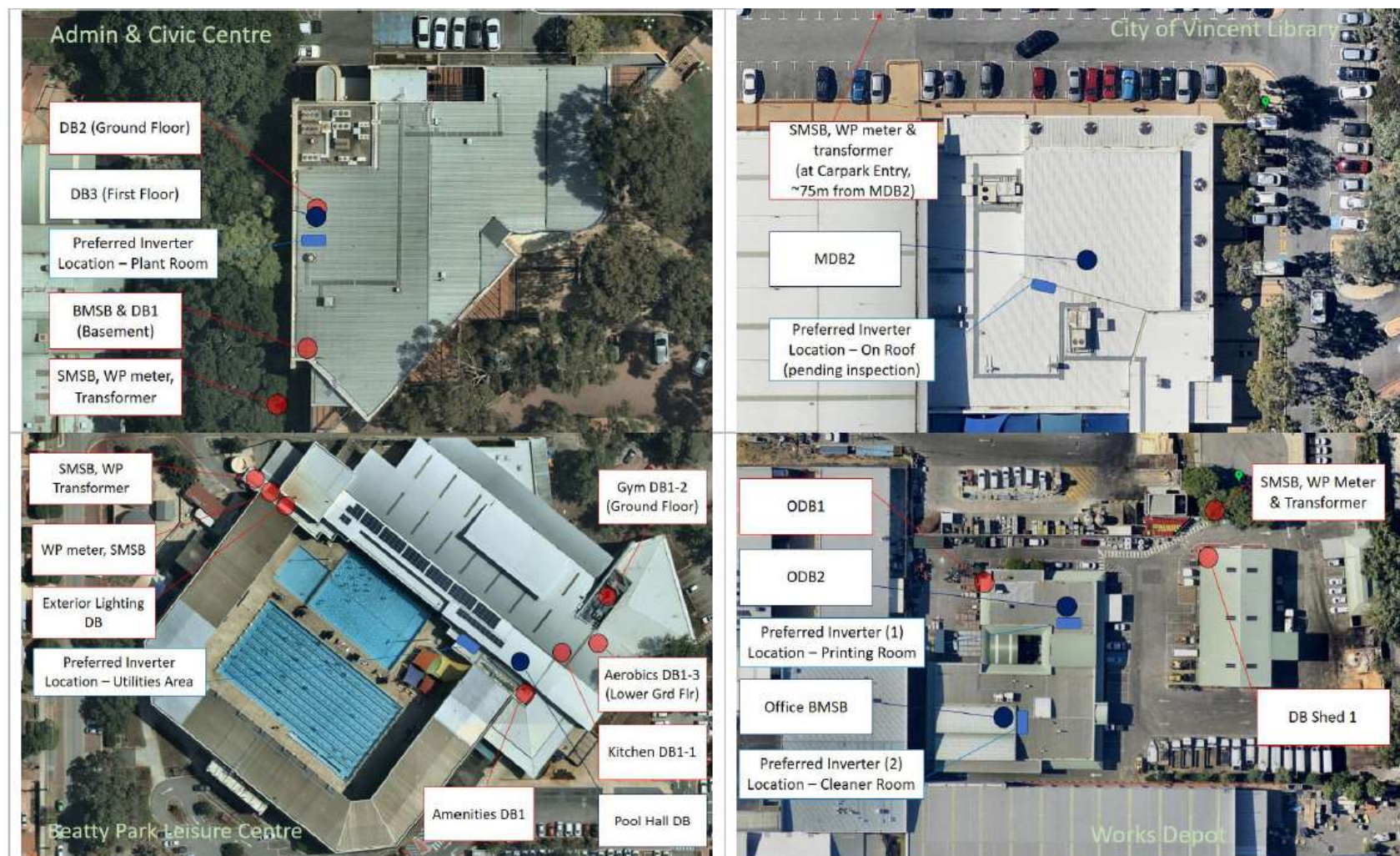
Figure 2 Existing electrical infrastructure and preferred inverter locations at the Administration & Civic Centre (top left), Beatty Park Leisure Centre (bottom left), the City of Vincent Library (top right) and the Works Depot (bottom right).
