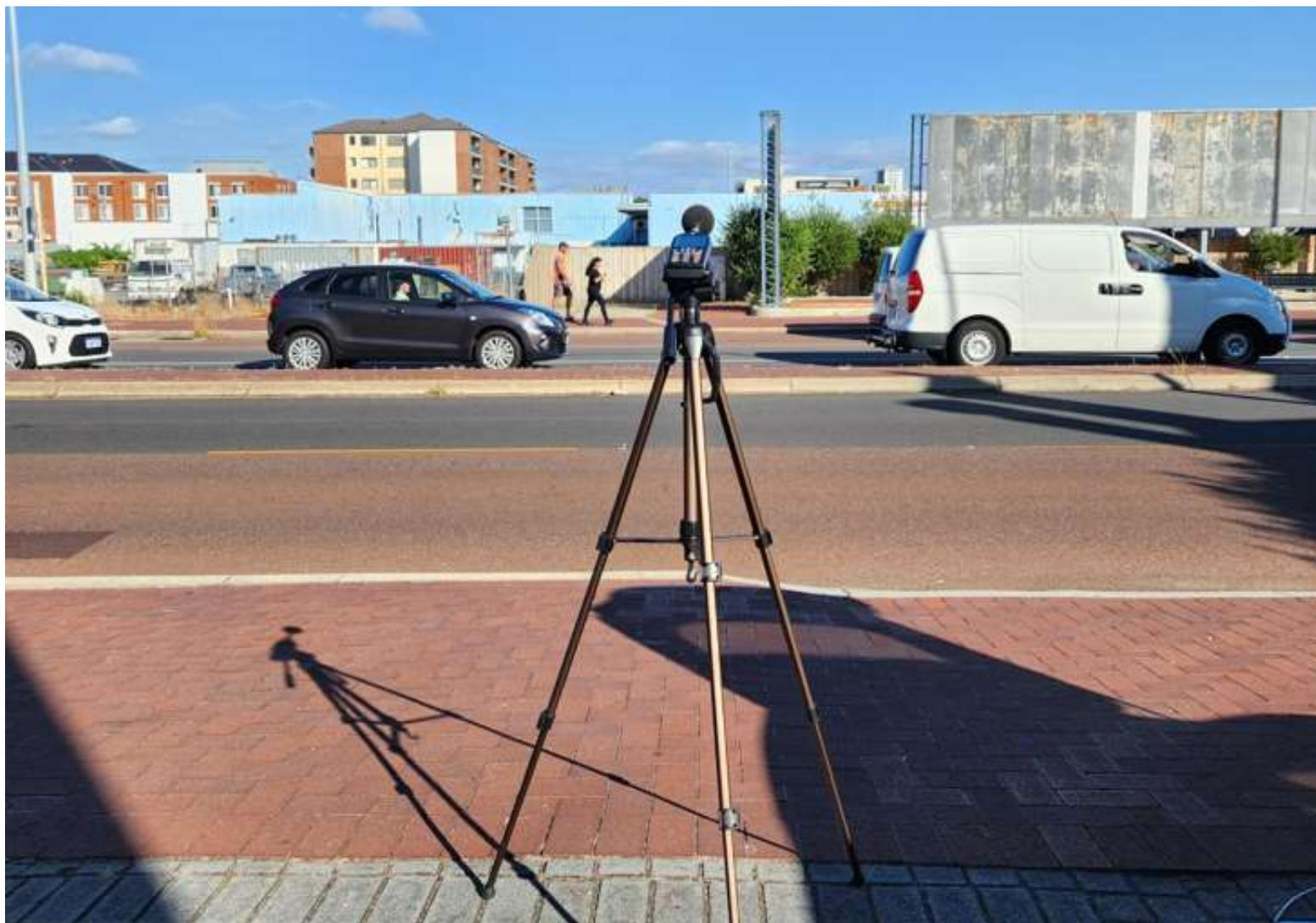
**Figure 4: Photo of the sound level meter.**
