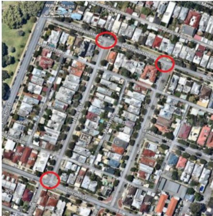
Treatments could consider mini roundabouts, raised plateau or seagull islands which considered with other proposed treatments, would work in allowing free flowing traffic, and not negatively impacting adjacent streets.
