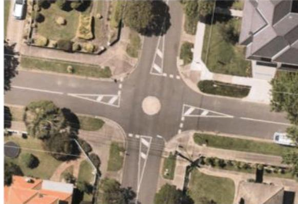
Figure 2: a typical mini roundabout in metropolitan Melbourne, Victoria
