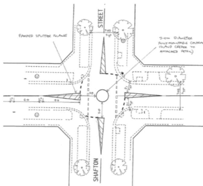
Figure 1 Plan drawing of mini-roundabout (Source: Tillotson 2015)
