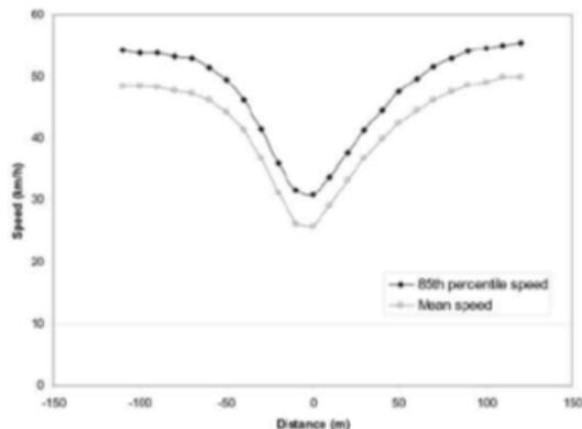
Figure C14 6: Typical speed profiles for centre blister islands
