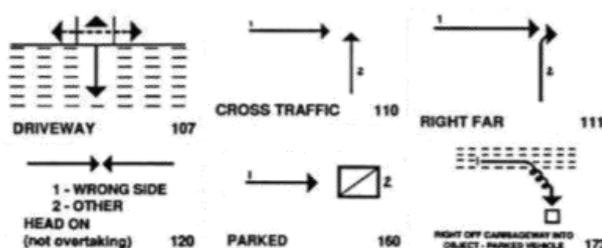
Figure 4 Relevant DCA crash diagrams (Source: VicRoads)
