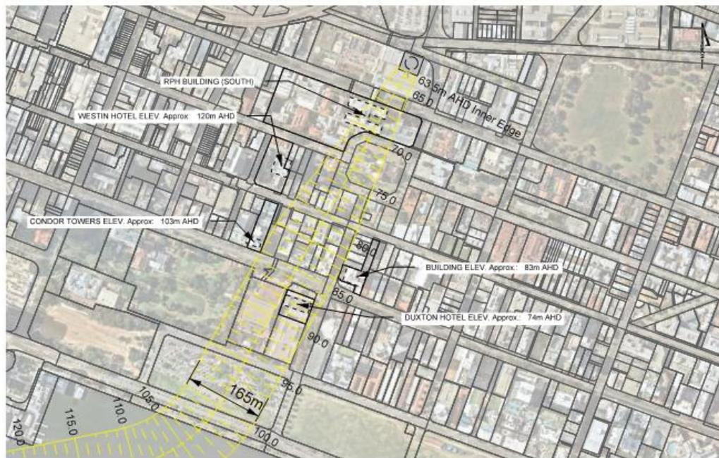
Figure 16. South west flight path and existing buildings
