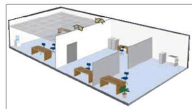
The principal element to consider in terms of maintaining separating wall Rw performance(s) and hence achieving practical levels of privacy and/or confidentiality in finished office spaces is therefore noise transmission passing over installed partitions via ceiling void space.
