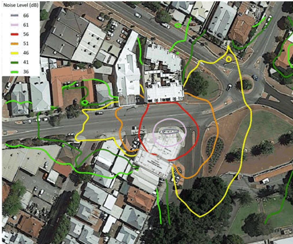
Figure 5 - Forecast  $L_{Amax}$  night-time noise contours @ 4.5m above ground
