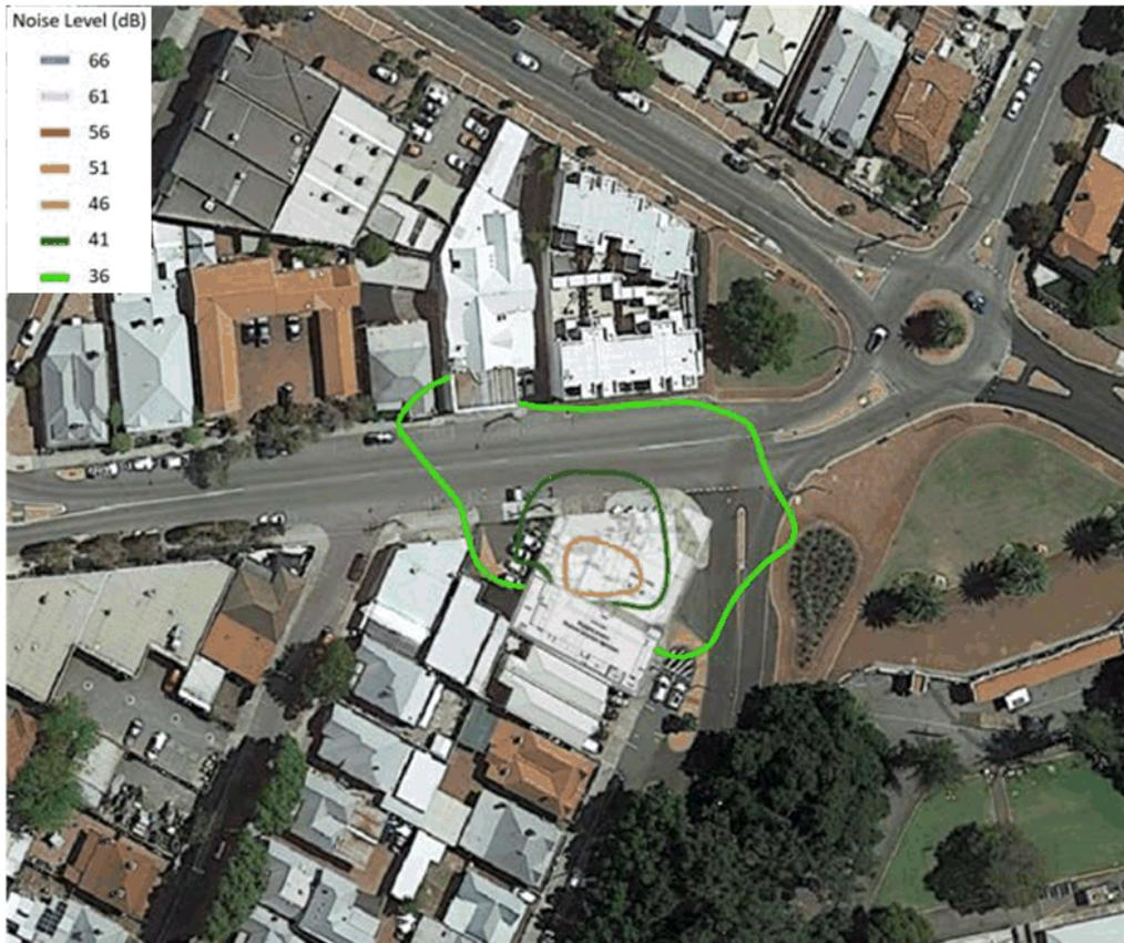
Figure 3 - Forecast  $L_{A10}$  night-time noise contours @ 4.5m above ground
