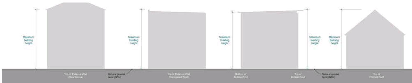
Figure 2 – 1.1 – Building Height Measurement
