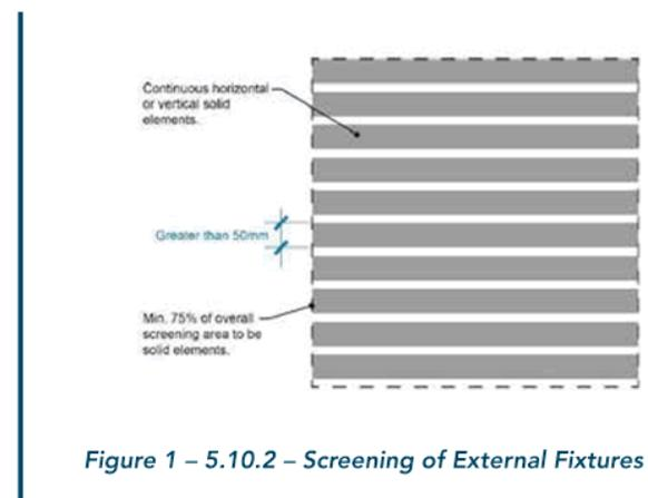
Figure 1 – 5.10.2 – Screening of External Fixtures
