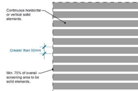
Figure 1 – 5.10.2 – Screening of External Fixtures
