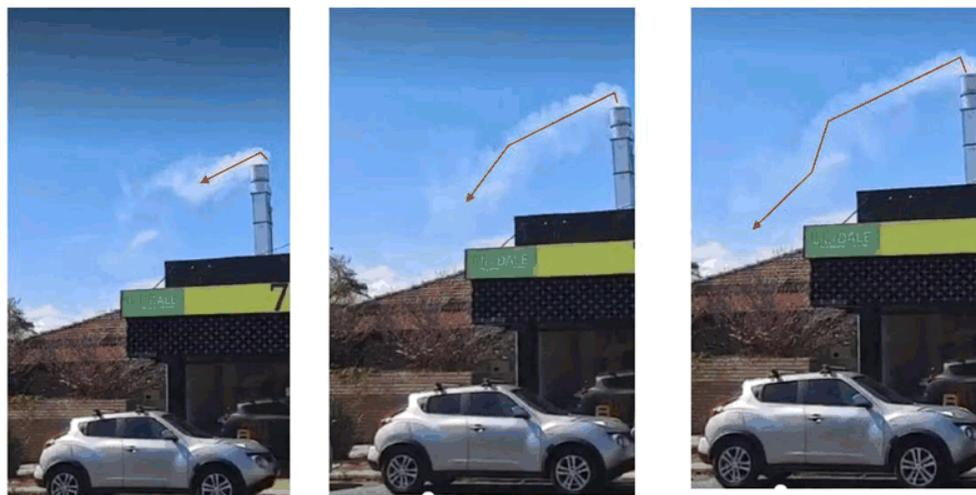
**Figure 13:** Sequence #1 – plume pushed down by downwash effect
