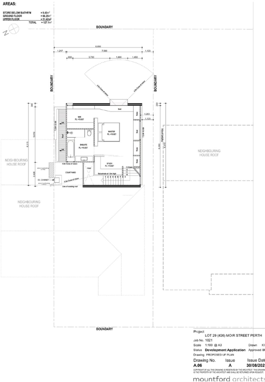
**FIGURE 9: PROPOSED UPPER FLOOR PLAN**
