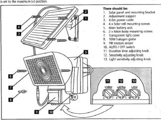
Once you have identified all parts, connect the solar charge panel to your Solar Security Light by plugging the 4.6m lead into the lead attached on the front of the Solar Security Light.
