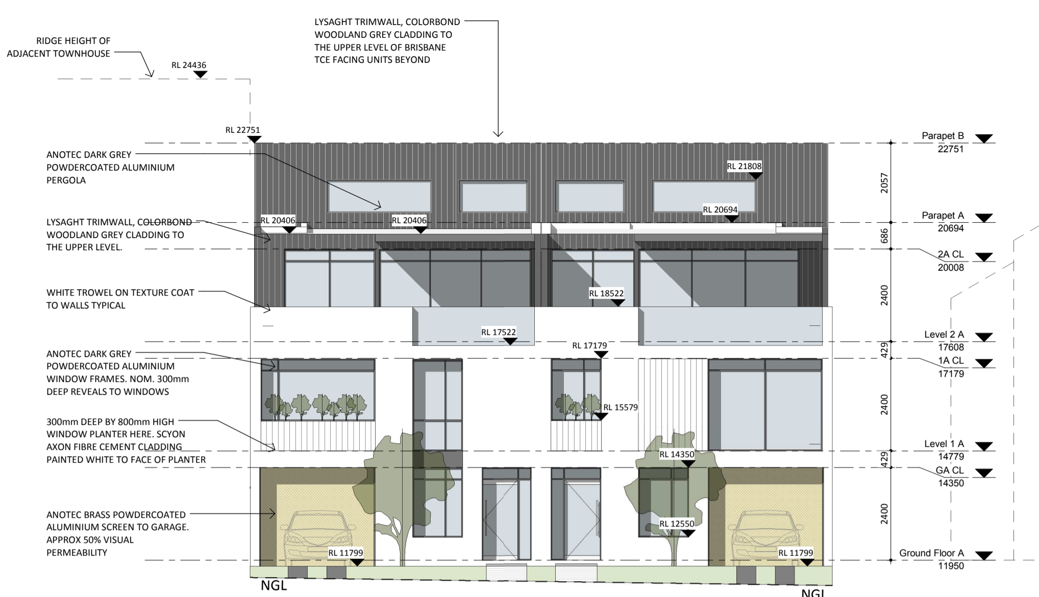
1 Robinson Ave (South) Elevation A01 1:100
