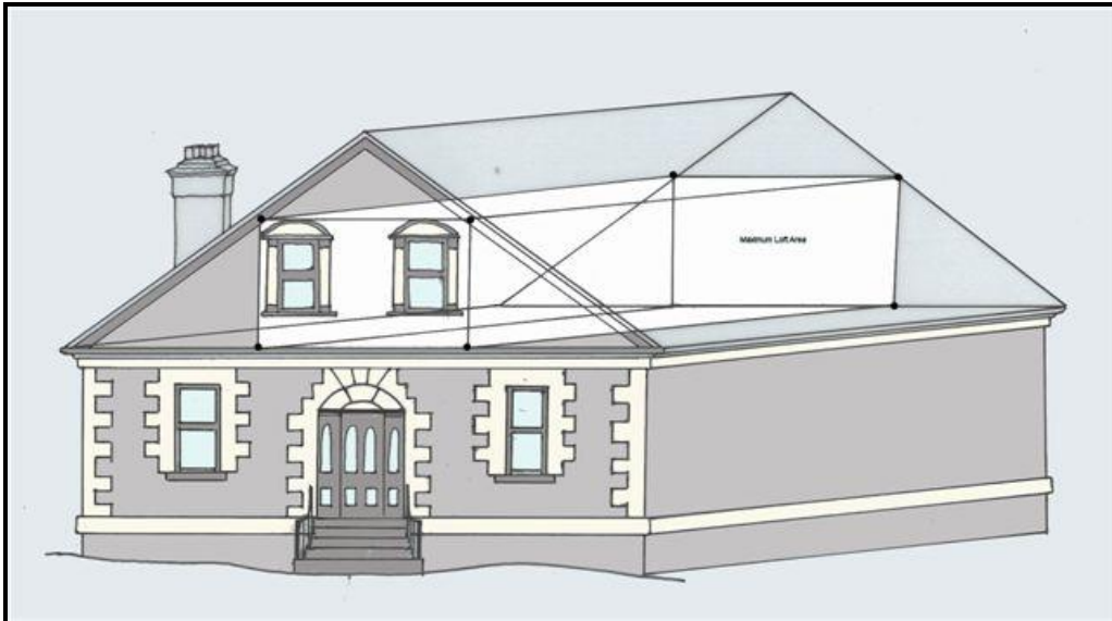
Figure 19: Loft Contained Within the Roof Space
