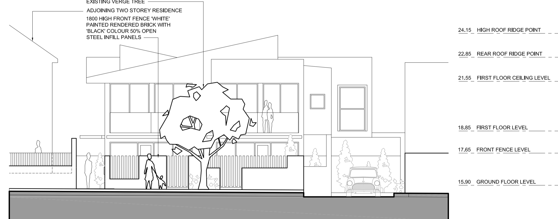
STREET (WEST) ELEVATION
