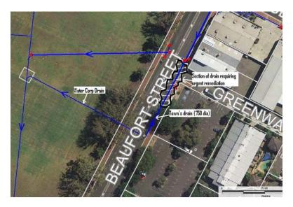
The Town's operations staff arranged for a camera to be sent down the pipe line and this revealed excessive infiltration of ground water and sediment at several locations. In addition when viewing the video footage it was clear that there was a surge in water ingress when a heavy vehicle passed over the drainage line.
