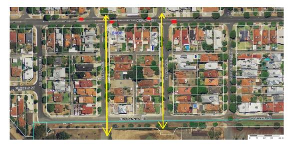
Anzac Road is classified as a District Distributor B in accordance with the Metropolitan Functional Road Hierarchy, has a posted speed limit of 50 kph, and provides a link between Oxford Street and Brady Street. The 85% speed is about 9 kph above the posted speed in some sections of the road. The Police have in past deployed traffic officers to monitor and enforce the 50 kph speed limit both as a visual deterrent and to change driver behaviour.
