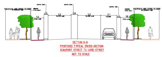
Figure 3. Cross- section of bike lane protected by parked cars
