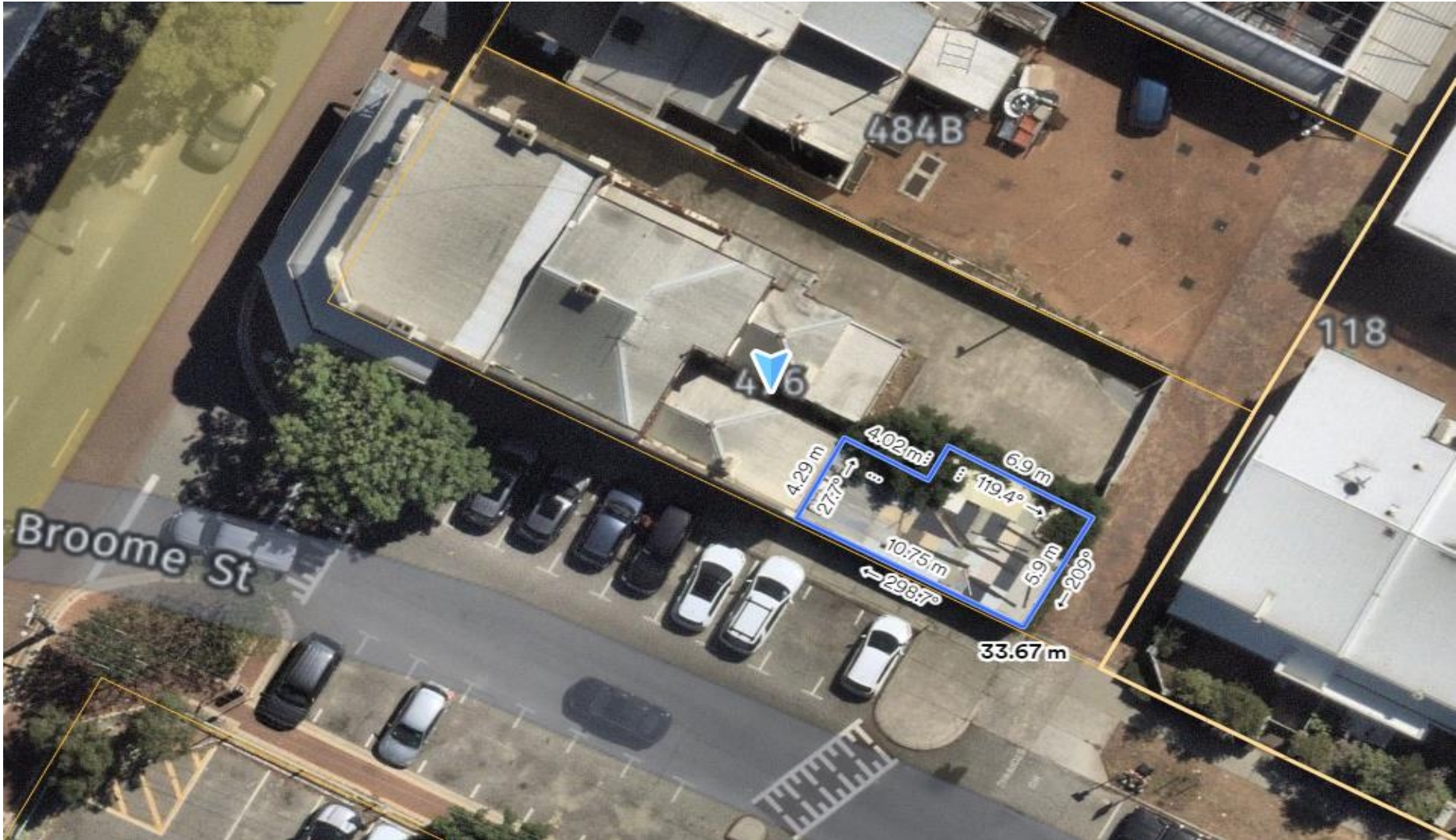
Removal of timber frame extension and brick toilet. Access /Egress from rear laneway. Manual separation from main building and load out with mini excavator.
