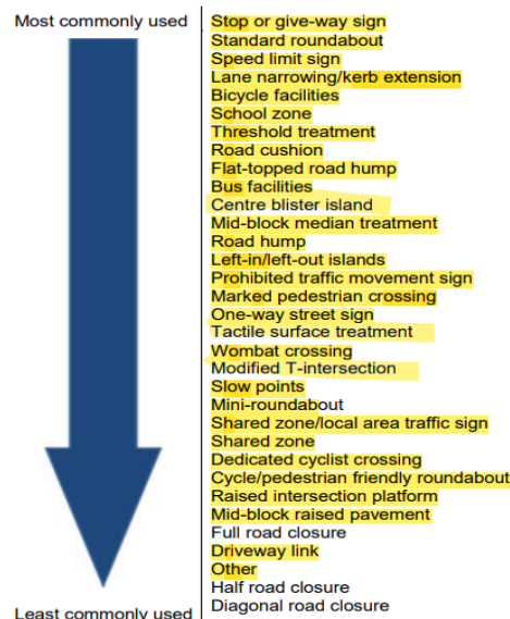
Figure 7.1: LATM devices commonly used by local governments
