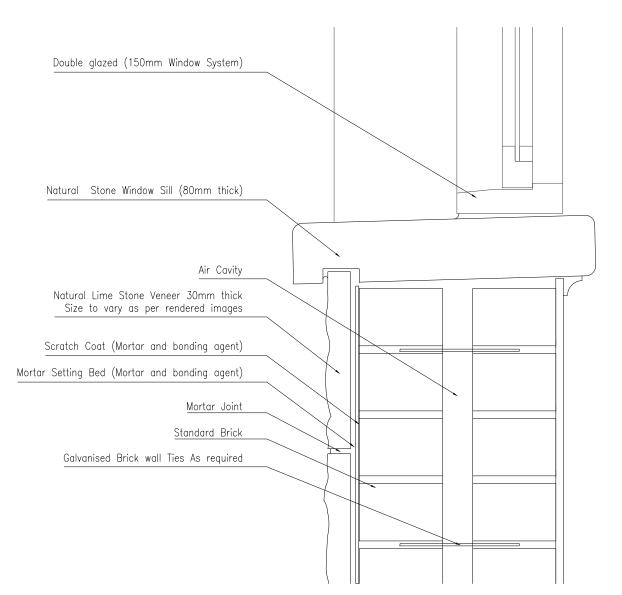
**Lime Stone Cladding Detail** Scale 1/5
