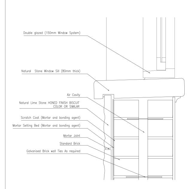
Lime Stone Cladding Detail Scale 1/5
