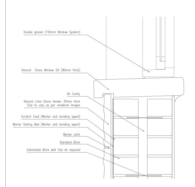
Lime Stone Cladding Detail Scale 1/5
