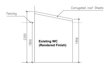
South elevation of WC SCALE 1:50
