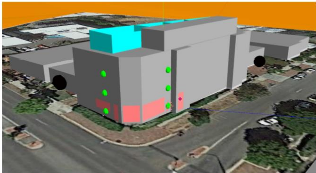
Figure 10 Noise model setup – Air conditioning units on the rooftop
