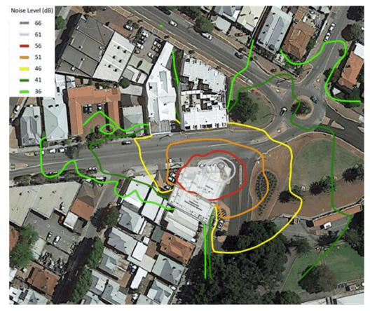
Figure 4 – Forecast L<sub>A1</sub> night-time noise contours@ 4.5m above ground (reduced volume tyre-refill beeper) (Residential Assigned Level = 51 dB)
