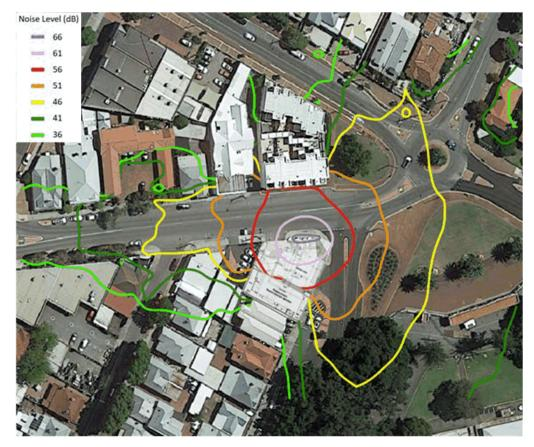
Figure 5 – Forecast  $L_{Amax}$  night-time noise contours @ 4.5m above ground (Residential Assigned Level =  $61\,\text{dB})$
