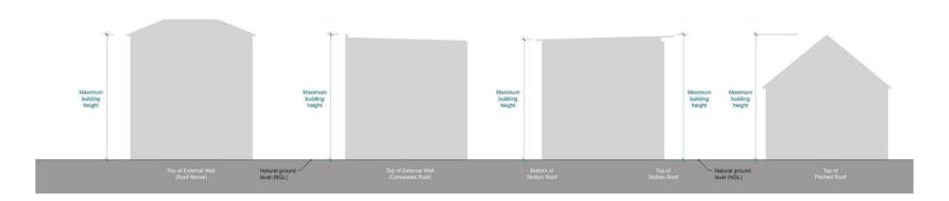
Figure 2 – 4.2 – Building Height and Measurement
