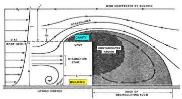
Fig. 1 Centerline Flow Patterns Around Rectangular Building 1,2
