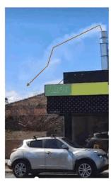
Figure 13: Sequence #1 – plume pushed down by downwash effect
