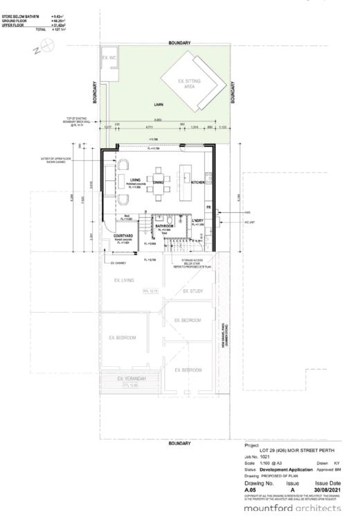
FIGURE 5: GROUND FLOOR PLAN OF PROPOSED TWO STOREY ADDITION
