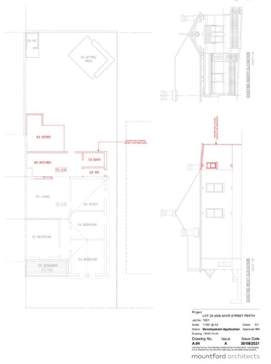
FIGURE 4: EXTENT OF DEMOLITION OF EXISTING HOUSE Courtesy: Mountford Architects
