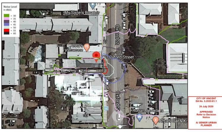
Figure 7: Worst-case noise contours at 1.5m above the ground.
