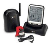
(Example of a Basic Energy Monitoring System, Current Cost model. Image source: www.diyhomeautomation.com.au)
