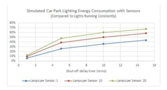
The simulation results shows that an energy saving of up to 90% can be achieved with well configured lighting controls. Three minute sensors with 10 lamps wired to a single sensor should deliver a 75% saving in run-time (6 hours per day run time verses 24 without any controls). Less lamps per sensor, or faster shut down will further reduce the runtime.
