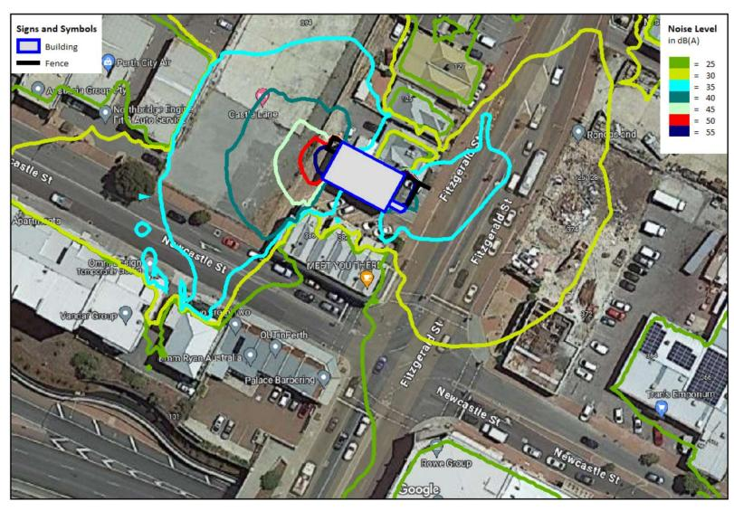
Figure 12: Worst-case noise contours at 1.5m above the ground for scenario 1.
