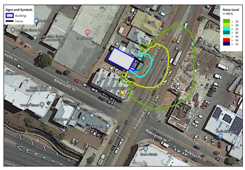
Figure 13: Worst-case noise contours at 1.5m above the ground for scenario 2.
