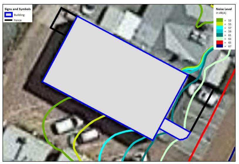
Figure 9: Day-time  $L_{Aeq(Day)}$  contours at 4.4m above the ground for current traffic flows.
