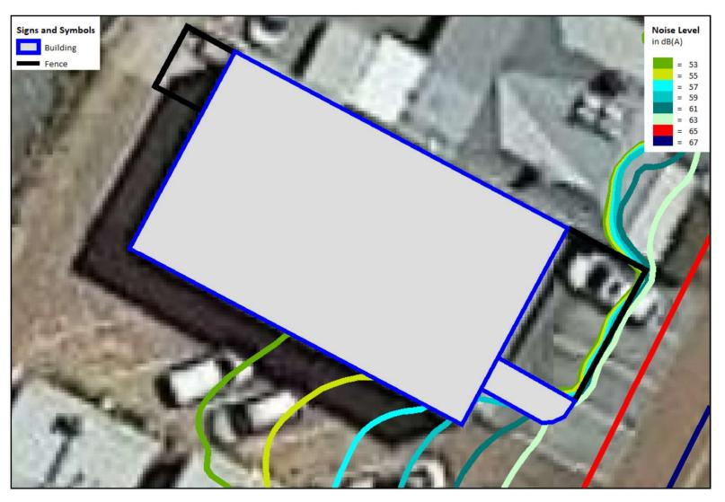
Figure 8: Day-time L<sub>Aeq(Day)</sub> contours at 1.4m above the ground for current traffic flows.
