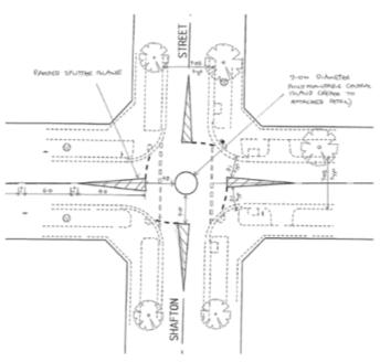
Figure 1 Plan drawing of mini-roundabout (Source: Tillotson 2015)
