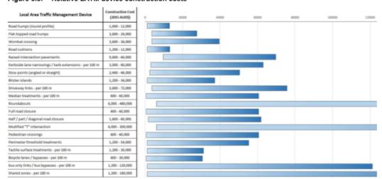
Figure 3.5: Relative LATM device construction costs
