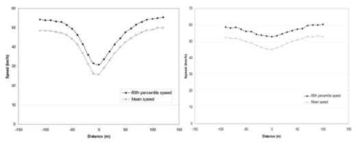
A linear relationship was developed (Austroads 2009b) for the minimum 85<sup>th</sup> percentile speed at a roundabout (V<sub>85min</sub>) as a function of its outer radius of the maximum travel path (Rmtp) as shown in the Equation C1 and Equation C2. The range of these radii found in the roundabout was 24 to 63 m.
