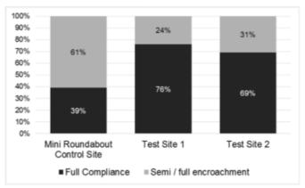
Figure 9 Driver encroachment over mini-roundabouts
