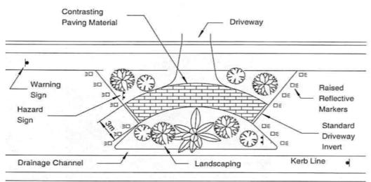
Figure 7.17: A typical driveway link treatment
