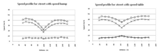
Legend: -O-: 85th Percentile speed. -X-: Mean speed. -A-: Standard deviation.
