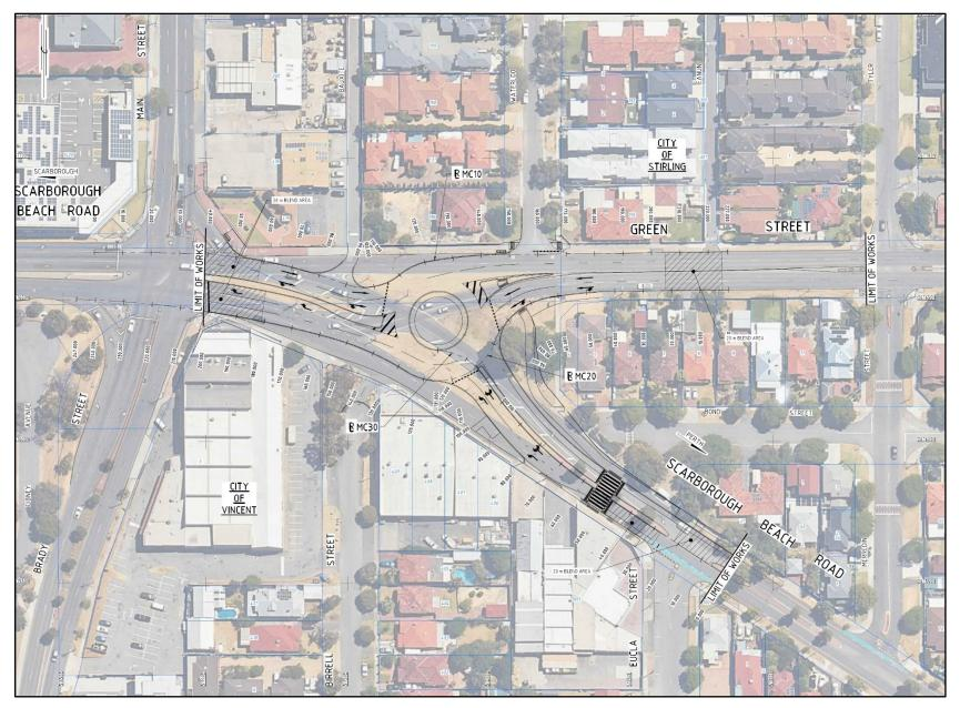
Figure 2 - Detailed Design Plan of Proposed Intersection Modifications
