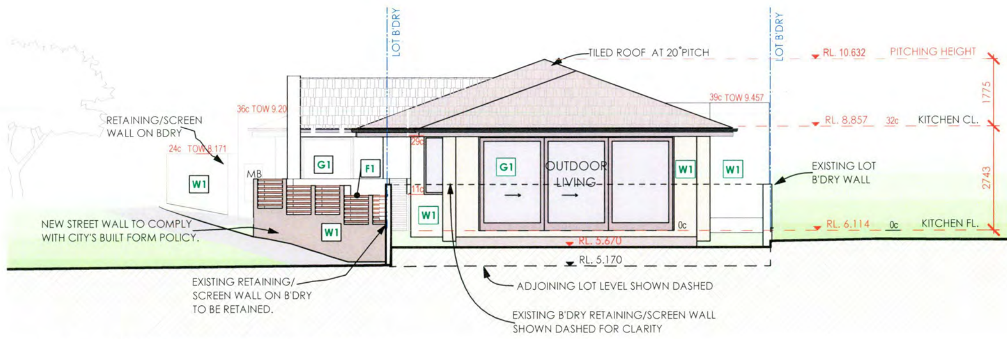
E4 DA.03 SOUTHERN ELEVATION SCALE 1:100 @ A3 SIZE
