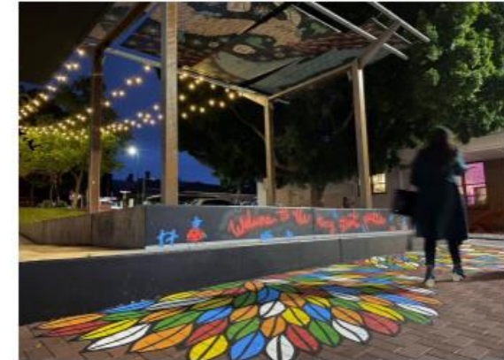
Mary Street Piazza corner is lit up and festoon lights provide good coverage. Kaadadjiny Laneway lights and wall gallery are connected to adjacent property and do not work when tenancy is vacant.
