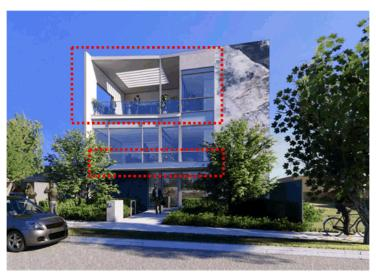
Figure 2.4 - Proposed shading devices
