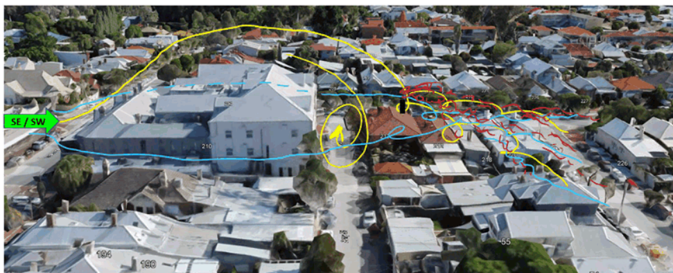
Figure 11: Grounding plume under a SE/SW wind
