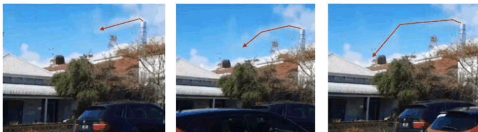
Figure 14: Sequence #2 – plume pushed down by downwash effect
