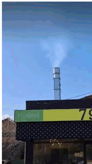
Figure 12: Vertical rise of the plume under no to very light wind
