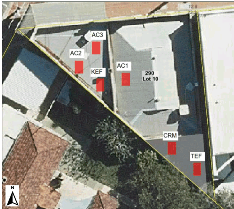
Figure 5.2.1: Proposed mechanical services roof plant.
