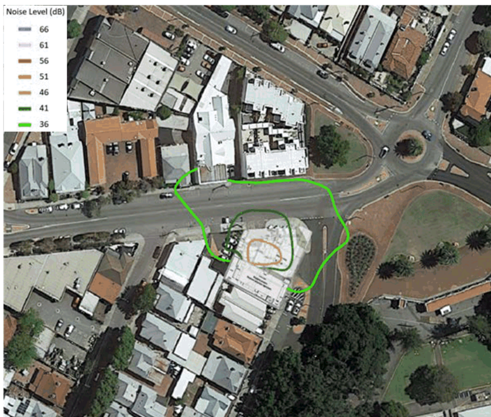
Figure 3 - Forecast LA10 night-time noise contours @ 4.5m above ground (Residential Assigned Level = 41 dB)
