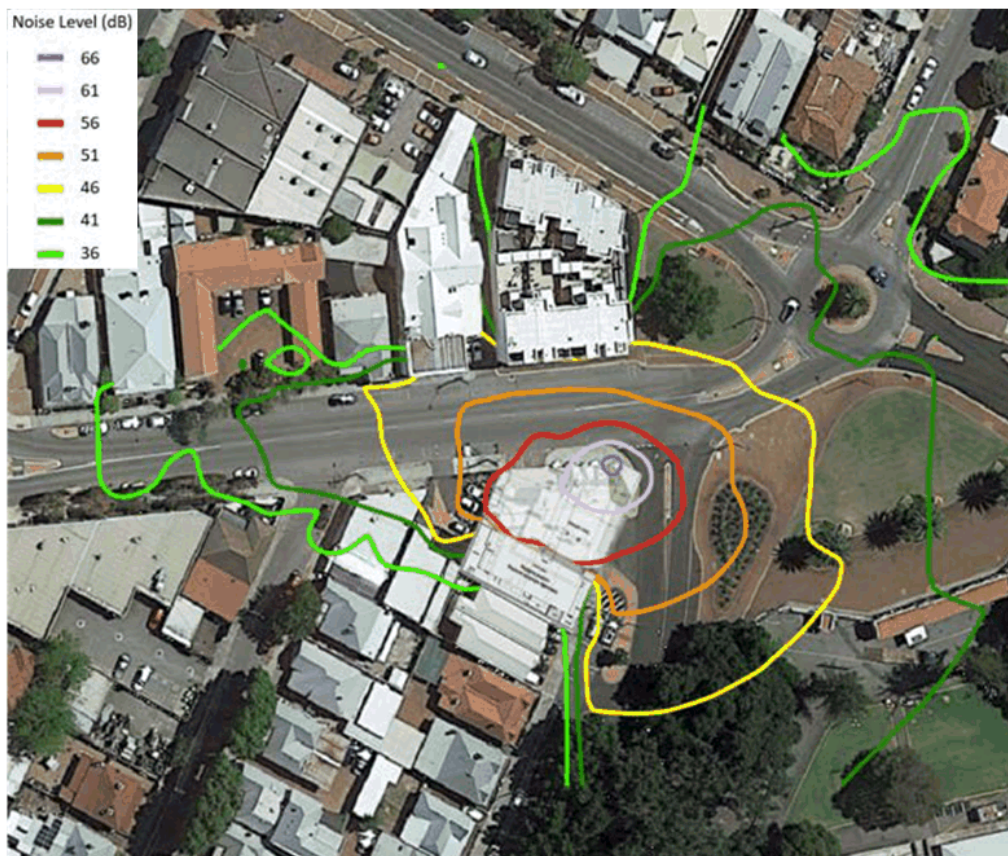
Figure 4 - Forecast L A1 night-time noise contours@ 4.5m above ground (reduced volume tyre-refill beeper) (Residential Assigned Level = 51 dB)
